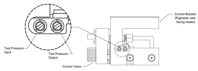
FIGURE 6. Pressure Test Point Location
